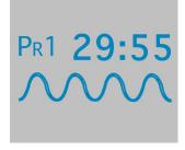
During operation, the controller displays the program that you have selected, the time remaining for your session and the waveform. The curved line indicates the program selected uses the sine wave. Programs using the square wave will display an animated square wave.
